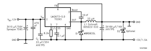
FIGURE 6. 5V to -15V/150mA Buck Boost Converter
