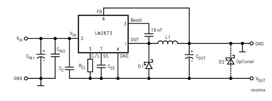
FIGURE 2. LM2673 Positive to Negative Converter
