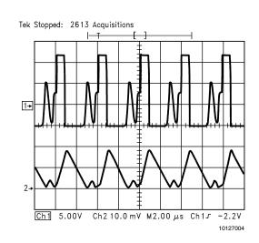
Upper Trace: Switch Voltage, 5V/div Lower Trace: Inductor Current, 0.5A/div Horizontal: 2µs/div
